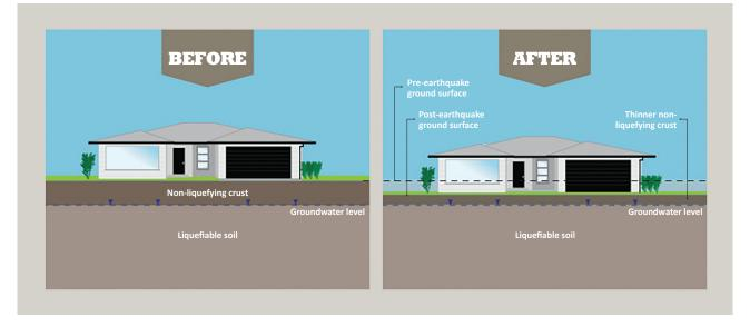
When an earthquake causes the land to subside, the non-liquefying crust of the land can become thinner. This effect is shown in the picture above.
