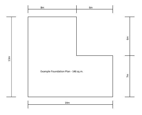
The treatment area for stone columns is the house footprint of 146m<sup>2</sup> plus a 2m perimeter, giving a total treatment area of 270m<sup>2</sup>.
