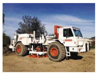
'T-Rex' - a shaker truck used for liquefaction shake testing
