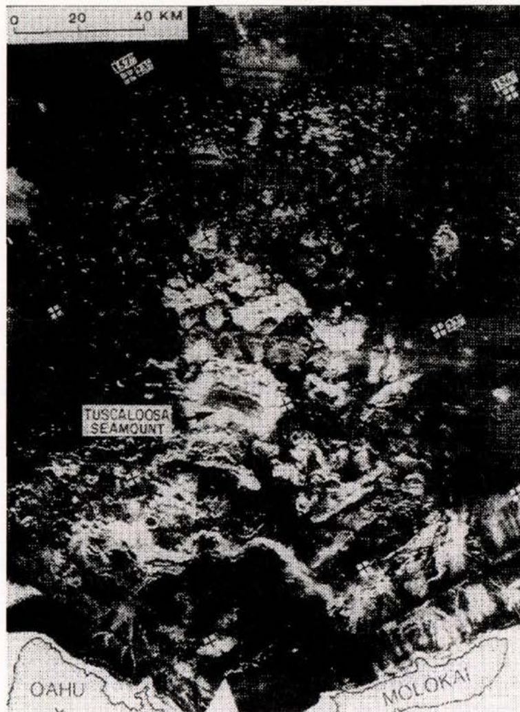
Figure 2.8. Side-scan sonar image of the Nuuanu (off Ohau) and Wailau (off Molokai) debris avalanches, Hawaii. Individual displaced blocks, the largest being the Tuscaloosa Seamount, appear as distinct light areas, generally becoming smaller away from the islands (Hampton et al. 1996).
