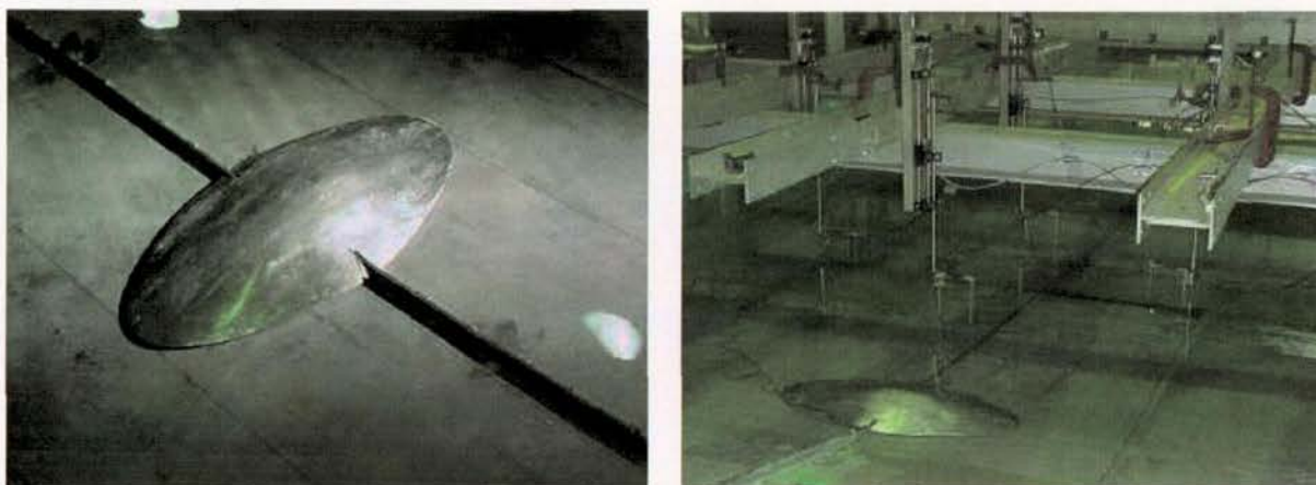
Figure 2.13. Photographs from the 3-dimensional tests of Enet et al (2003). The photo on the left shows the flattened dome-like model landslide mounted to a guiding rail. The photo on the right shows the array of capacitance wave gauges, used to measure wave heights, placed over the wave tank.
