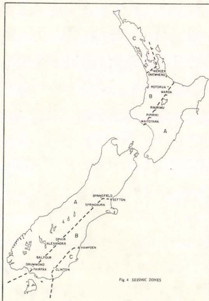
(b) Seismic Zones - Fig. 4, NZS 4203: 1984
