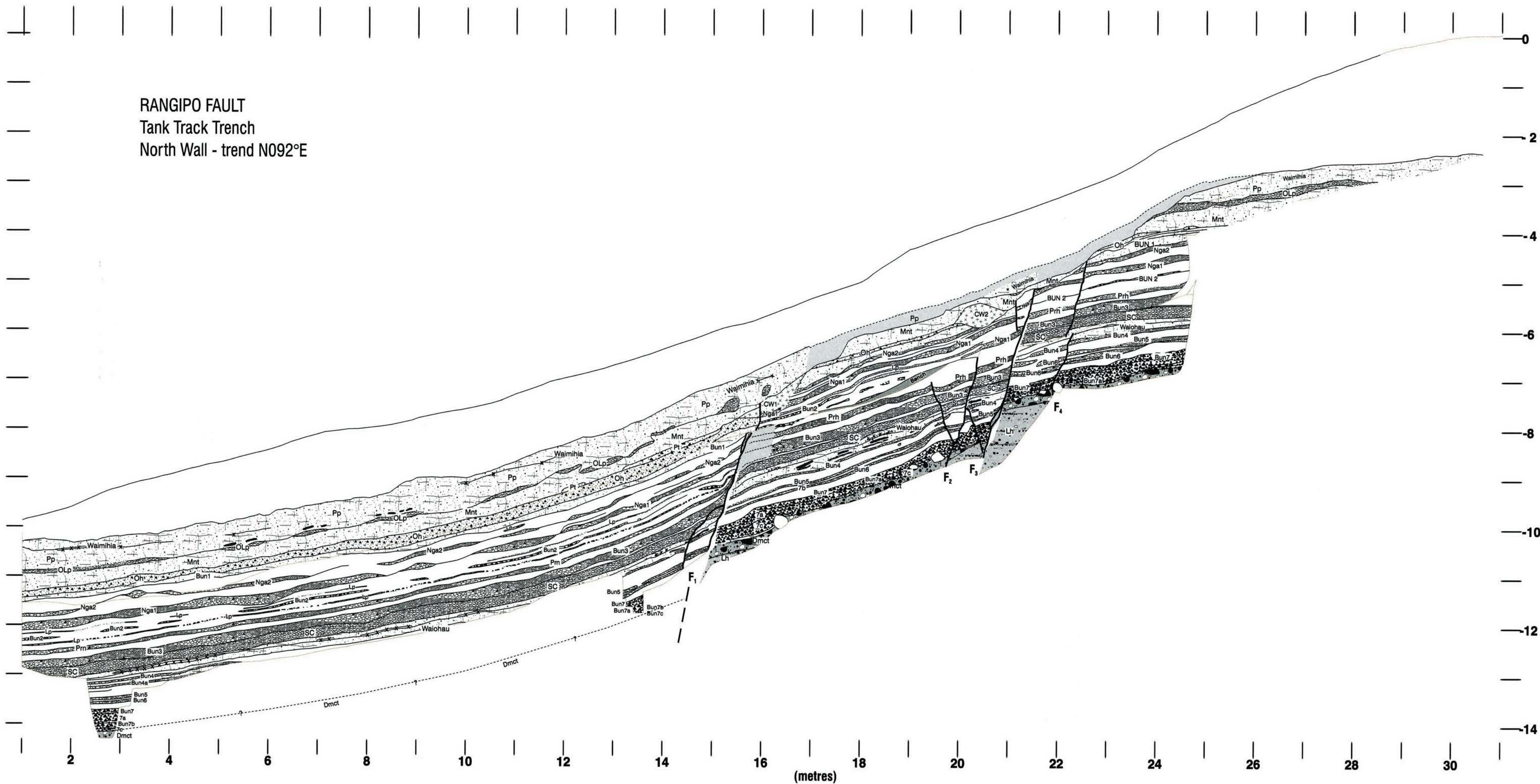
Figure 3.15C) Restoration of the base of the Papakali Tephra, Tank Track Trench log.
