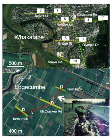
**Figure 4.1** Overview of the survey area and seismic profiling map (yellow lines) at Edgecumbe (lower) and Whakatane (upper) survey sites. At Edgecumbe, the red dotted line marks the fault scarp of the 1987 rupture, the green dotted line marks the linear extrapolated Whakatane Fault trace from its known location south of the city. Street names: 1 - McCracken Rd, 2,3 - farm tracks, 4 - Goulstone Rd, 5 - Stewart St, 6,7 - James St, 8 - Bridge St, 9 - Olympic Dr, 10 - Arawa Rd, 11 - Gorge Rd.
