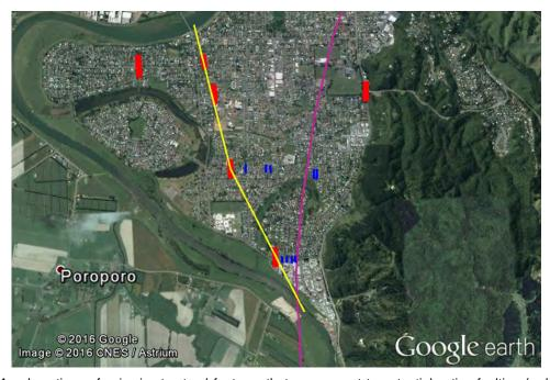
**Figure 7.1** Locations of seismic structural features that we connect to potential active faulting (red markers). The blue markers show positions of other small offsets of seismic reflection horizons we've observed in the data. The yellow line connects four of the features observed on individual profiles. The purple line shows the approximated location of the Whakatane fault as it is currently given in the Active Fault Database (Langridge et al., 2016).
