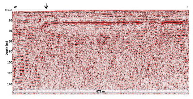
**Figure 5.11** Depth section of profile 5 in Whakatane township based on velocities derived from the seismic data only and with a horizontal-to-vertical scale of 1:2. The depth range of seismic reflectivity achieved is up to 100 m, the mean velocity is nearly 200 m/s. Topographic corrections are applied using 33 a.s.l. reference datum. See Figure 4.1 for profile location.
