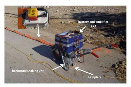
**Figure 4.2** Wheel-barrow mounted vibratory shear wave seismic source system developed by LIAG. The electrodynamic driven shaker unit is mounted in the aluminium casing below the blue box, which contains the batteries and the amplifier unit. The analogue signal used for the shaking control is sent via the yellow wire from the operators place in the recording car. Small photo: horizontal geophone unit mounted on a skid system.
