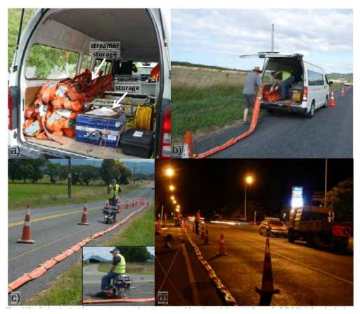
**Figure 4.3** Seismic land streamer receiver system (developed by LIAG and GEOSYM): a) during transportation including the dismounted source system; b) during release on site; c) during recording operation on Edgecumbe Fault slope site; d) during night operation in Whakatane. The geophone system was permanently connected to a GEODE seismic recording unit of 96 channels within the recording car at the front of the streamer, from where the recording operation was managed.
