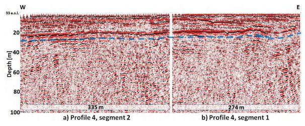
**Figure 6.2** Depth sections of profile 4 with a horizontal-to-vertical scale of 1:2 (each). The profile was acquired in two segments (2, west, 1 east) along Goulstone Rd. The profile clearly exhibits a marker horizon (blue dashed line traces the horizon slightly deeper to avoid concealing it), which correlates well with findings in Begg et al. (2015)( see Figure 6.3). Figure 4.1 provides profile location.
