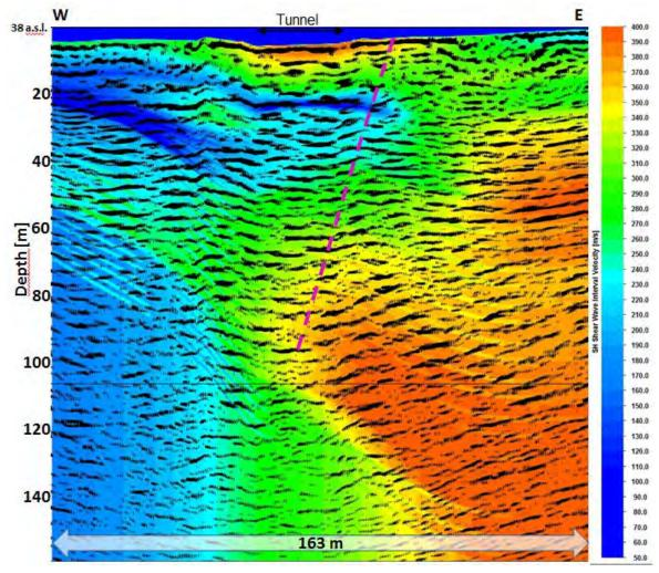
**Figure 6.11** Shear wave interval velocity structure for profile 11 (compare with Figure 6.10). The dashed magenta line gives a tentative interpretation of a potential fault location which was expected due to the geological structure. This profile was acquired through the pedestrian tunnel made of concrete connecting Goulstone Rd and Gorge road. The location of the tunnel is indicated and also visible due to the high velocities close to the surface. See Figure 4.1 for profile location.
