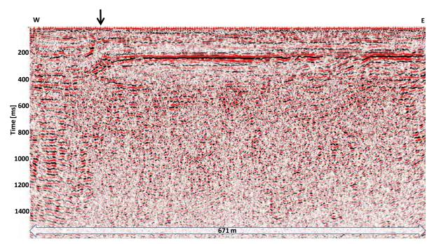
**Figure 5.10** Resulting time section of the FD-time migration process along profile 5 in Whakatane township. FD-time migration eliminates residual diffractions and corrects the position of dipping structures. See Figure 4.1 for profile location.
