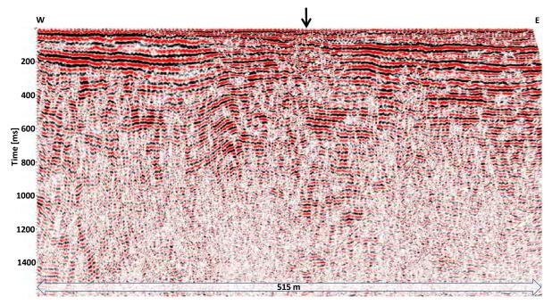
**Figure 5.4** Resulting time section of profile 1 (Edgecumbe Fault) after FD-time migration to eliminate residual diffractions and to correct positions of dipping structures. Compared to Figure 5.3 the effect of this process is only small, which is mainly caused by the low velocities. The result of the process is also an indicator of quality to see whether the velocity field matches the data field. Topographic corrections are still not applied. See Figure 4.1 for profile location.
