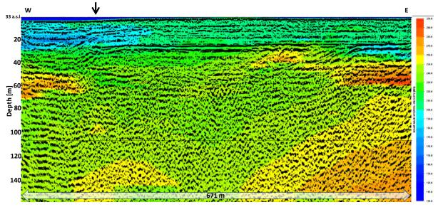
**Figure 5.12** Depth section of profile 5 in Whakatane township colour coded by shear wave interval velocities in depth derived from the seismic data (horizontal-to-vertical scale of 1:2). Due to the limited offset range of the survey setup, velocities below 80 m may be erroneous. The blue zone on top left is caused by topographic corrections applied (reference datum 33 m a.s.l.). See Figure 4.1 for profile location.
