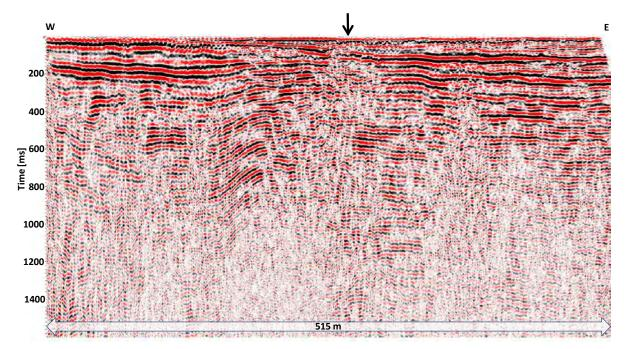
**Figure 5.3** Resulting time section of profile 1 (Edgecumbe Fault) after application of FX-deconvolution used for lateral frequency alignment. The position of the surface scarp of the fault is indicated by the black arrow and the fault dips steeply (~70°) to the west (W). See Figure 4.1 for profile location.
