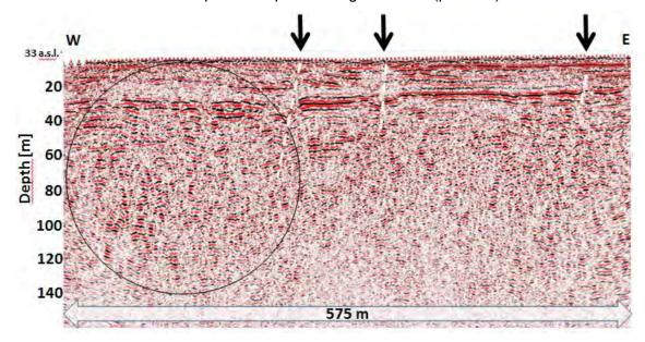
**Figure 6.7** Depth converted migrated section of profile 8 along Bridge Street, Whakatane. Note the continuous reflection of the marker horizon nearly 20 m depth below surface in the east that is interrupted at least twice (arrows). It becomes less continuous to the West (circled area) where also dipping structures and increased scattering occur below the marker horizon. The dashed white lines are interpretations of faulting on this profile. See Figure 4.1 or profile location.
