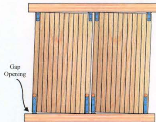
Figure 4: Deformed shape of the proposed concept for CLT platform structure with slip friction connections
