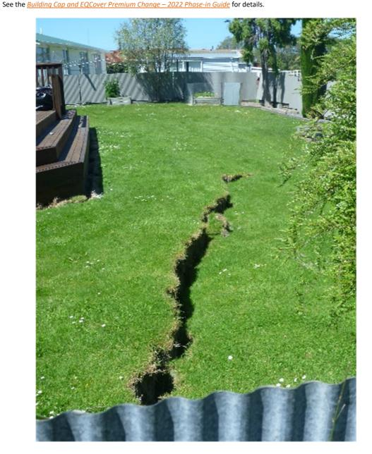
Figure 33 Cracking (lateral spreading) due to earthquake
