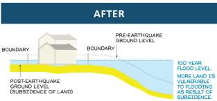
The above diagram shows how ground subsidence from the Canterbury earthquakes has made some properties more vulnerable to flooding.
