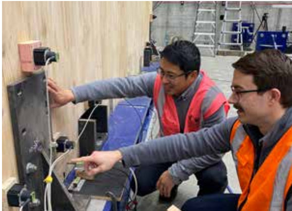
DR MINGHAO LI (LEFT) AND BEN MOERMAN CHECK THE CLT WALL TEST SET UP.
