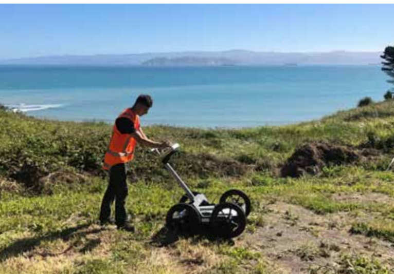
LEFT: MATT COOK USES GROUND-PENETRATING RADAR TO INVESTIGATE A POTENTIAL LANDSLIDE IN GISBORNE. RIGHT: DR MURRAY CAVE ON A ROCKSLIDE AT MANGAPOIKE NEAR GISBORNE.
