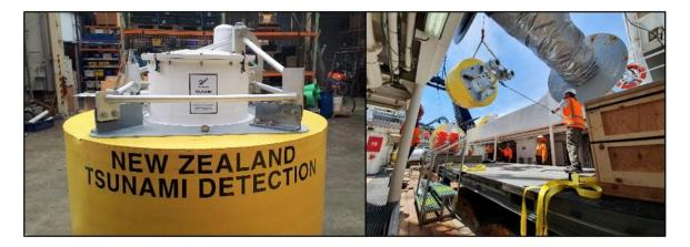
DART buoys have sensors on the seafloor that measure changes in water pressure. Buoys at the surface send signals via satellite to the National Geohazards Monitoring Centre to warn of rapid changes signifying tsunami generation. Buoys are currently being deployed around New Zealand from NIWA's research vessel Tangaroa. Photos courtesy GNS Science's twitter account.
