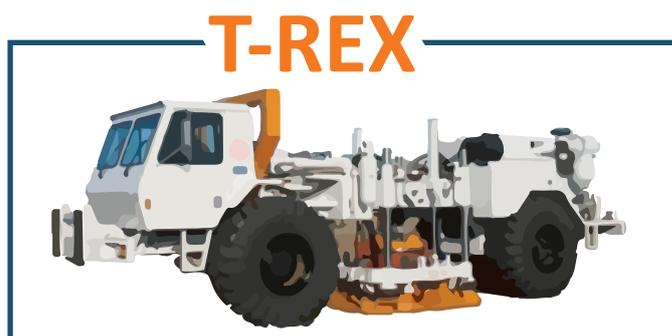
The T-Rex truck uses a large metal plate to create intense, but highly localised, shaking that diminishes rapidly with increasing distance from the truck. This shaking is applied to areas of test site land to assist in the evaluation of the strengthening methods being trialled.
