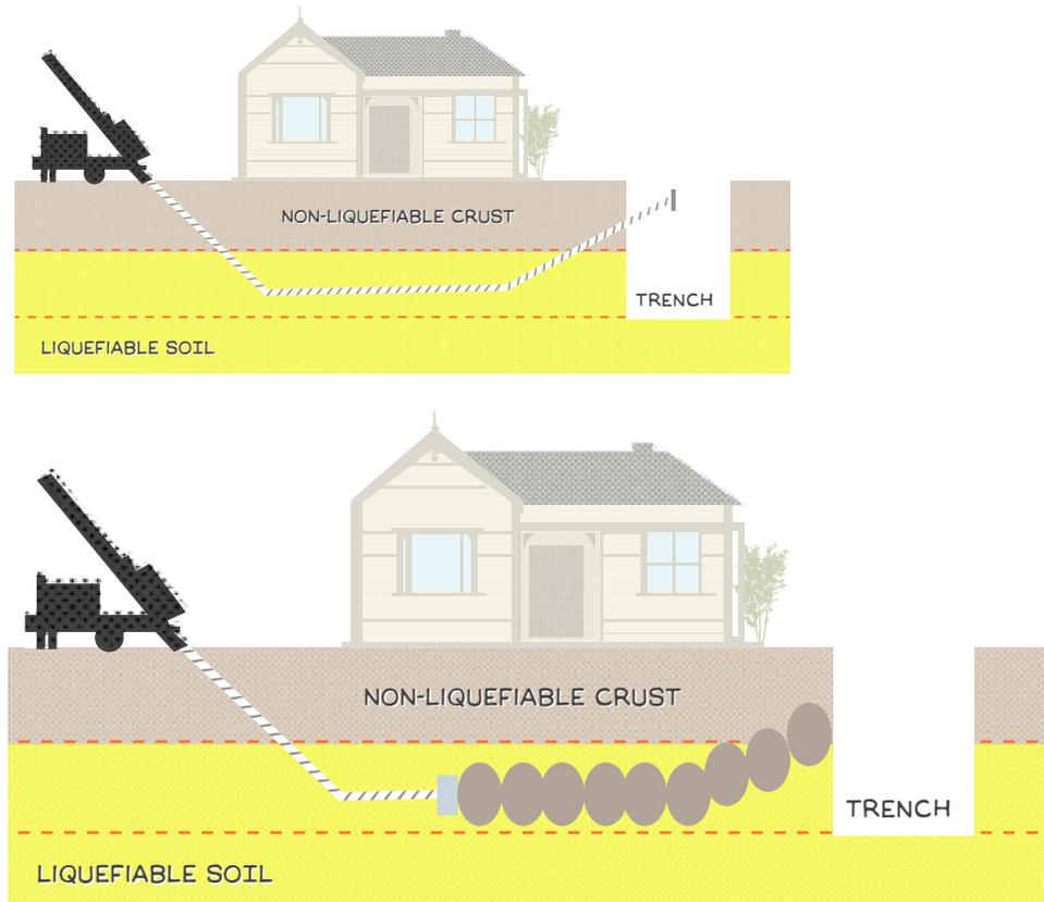
This technique offers advantages in situations where an existing building is to remain in place or where vibration and space constraints exist due to close proximity to neighbouring properties.
