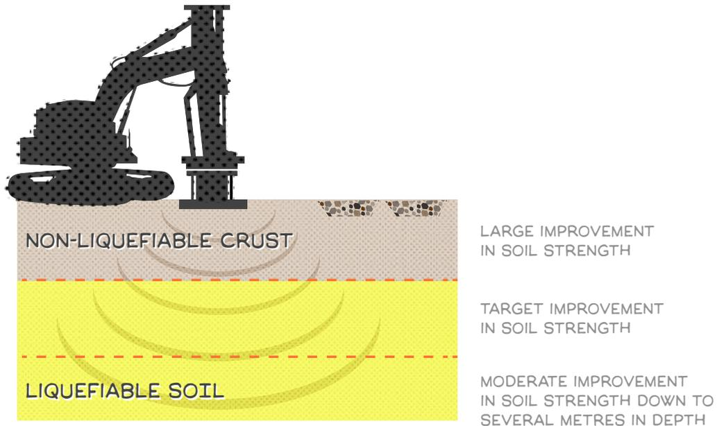
RIC is a smaller-scale version of a method called Dynamic Compaction which has been widely used on projects in New Zealand and around the world. It was used in the foundation work of Te Papa Museum in Wellington, for example.
