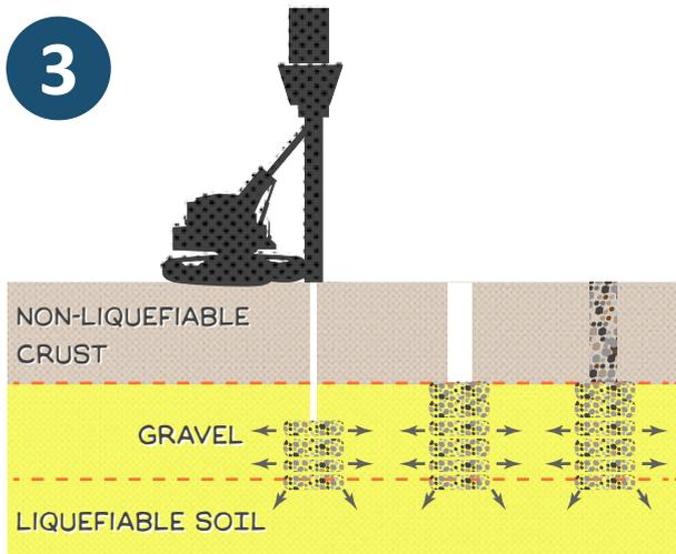
Working on a similar principle as the LMG method, this technique uses gravel, instead of concrete, to create columns that help stiffen the soil. A mandrel is pushed into the ground with a very powerful hydraulic ram, down to the target improvement depth. Gravel is fed down the hollow stem of the mandrel and released into the ground at depth.
