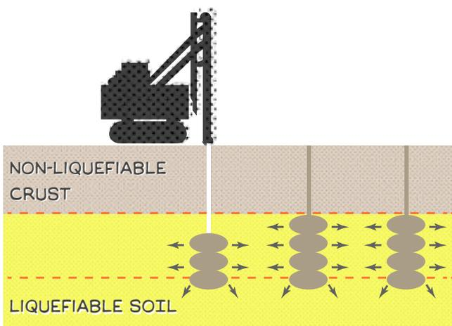
Also known as Compaction Grouting, this method works by injecting low-mobility (concrete consistency) grout to form a column of concrete “bulbs” within the soils. This squeezes out the existing soil sideways, providing densification and a positive increase in horizontal soil stresses, while the concrete columns also provides a stiffening of the soil.
