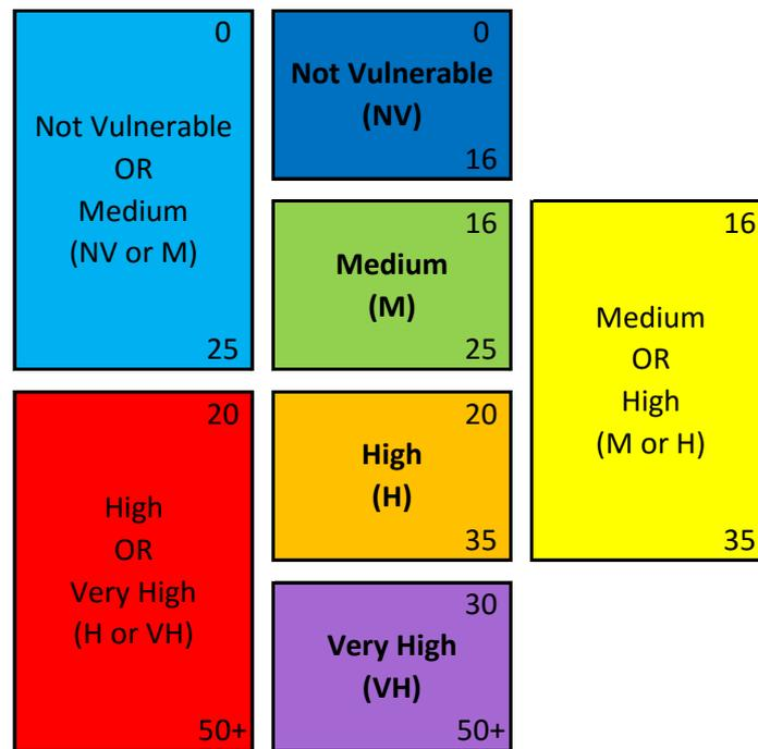
Figure A2.1: The **pre-CES** and **post-CES** liquefaction vulnerability severity classifications, divided into four primary classifications (in bold) and three 'OR' classifications with the range of LSN values for each classification indicated in the bottom and top right hand corners of the boxes.
