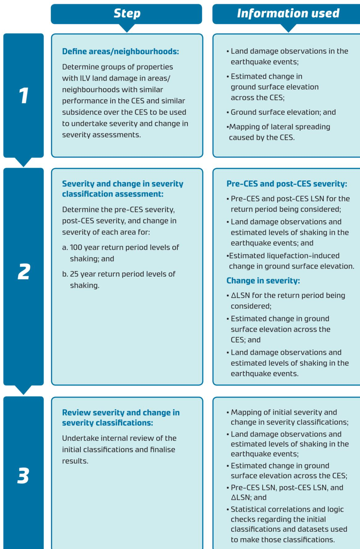
Figure A3.1: Overview of the ILV severity and change in severity classification manual process.
