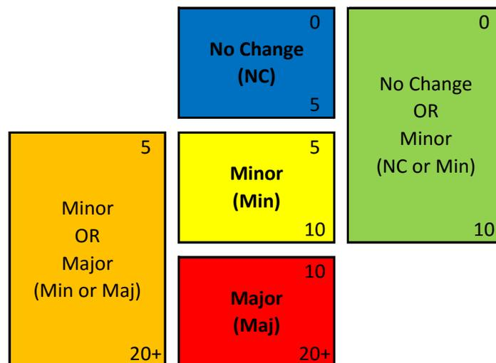
Figure A2.2: The extent of **change** in liquefaction vulnerability severity from **pre-CES** to **post-CES** divided into three primary classifications (in bold) and two 'OR' classifications with the range of change in LSN values for each classification indicated in the bottom and top right hand corners of the boxes.
