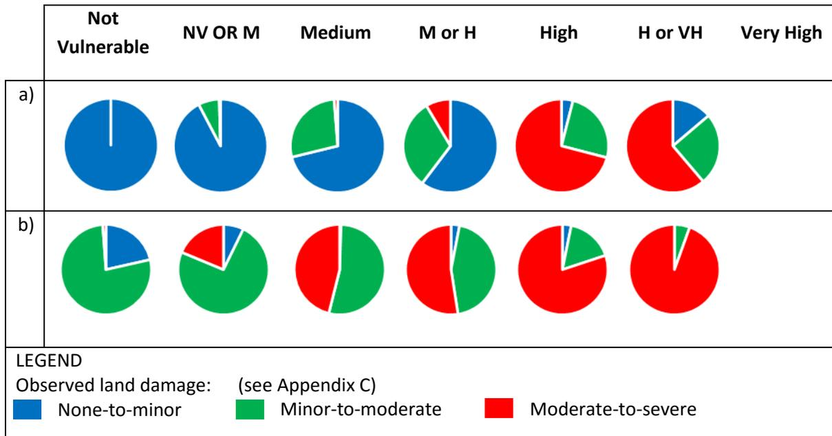
Figure A3.2: Statistical correlation of pre-CES liquefaction vulnerability severity classifications of properties with ILV land damage at 100 year return period levels of shaking with a) observed land damage following the September 2010 event and b) worst observed land damage during the CES.
