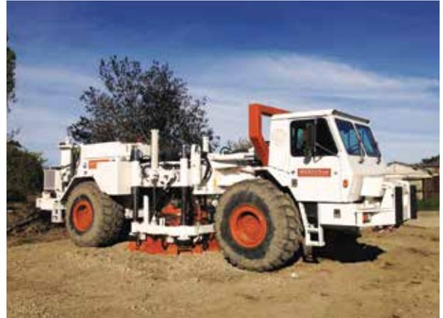
'T-Rex' – a shaker truck used for liquefaction shake testing
