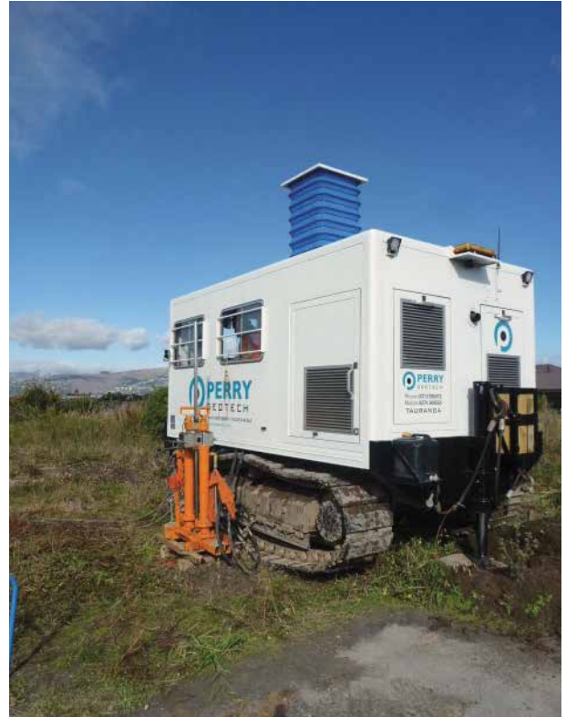
A cone penetration test
