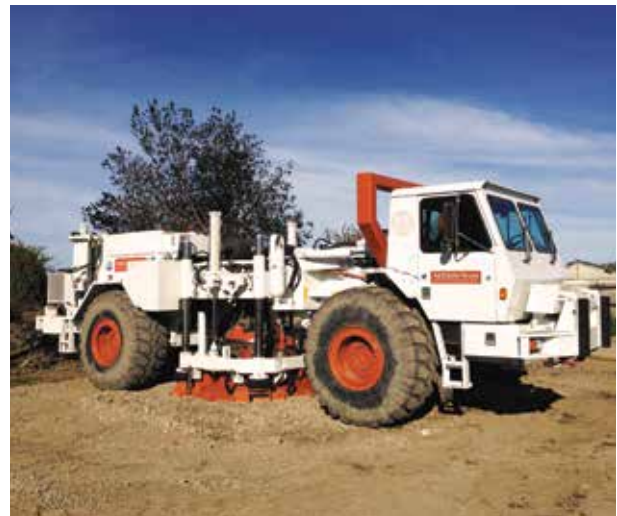
T-Rex – machine for liquefaction triggering testing
